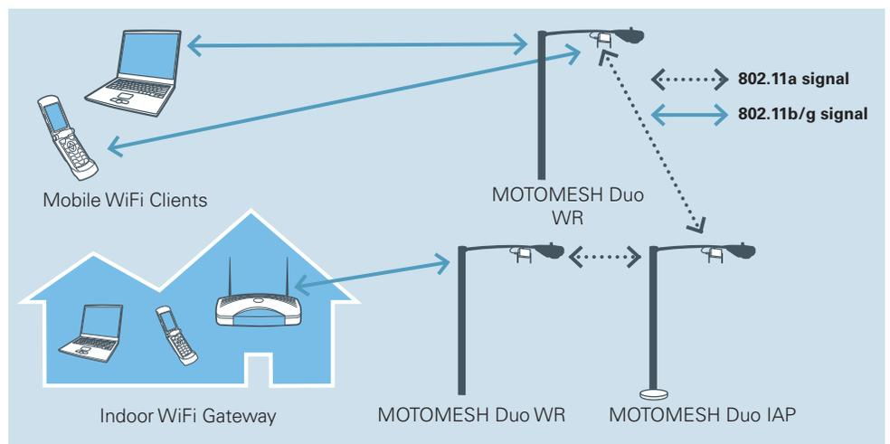
There are benefits to each of the configurations, and decisions should be made based on user requirements. The two radio configuration can improve overall network throughput, reduce latency and enable more clients to be served by a single backhaul link.
