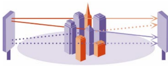
MIMO minimizes signal fading due to path obstructions or atmospheric disturbances.
